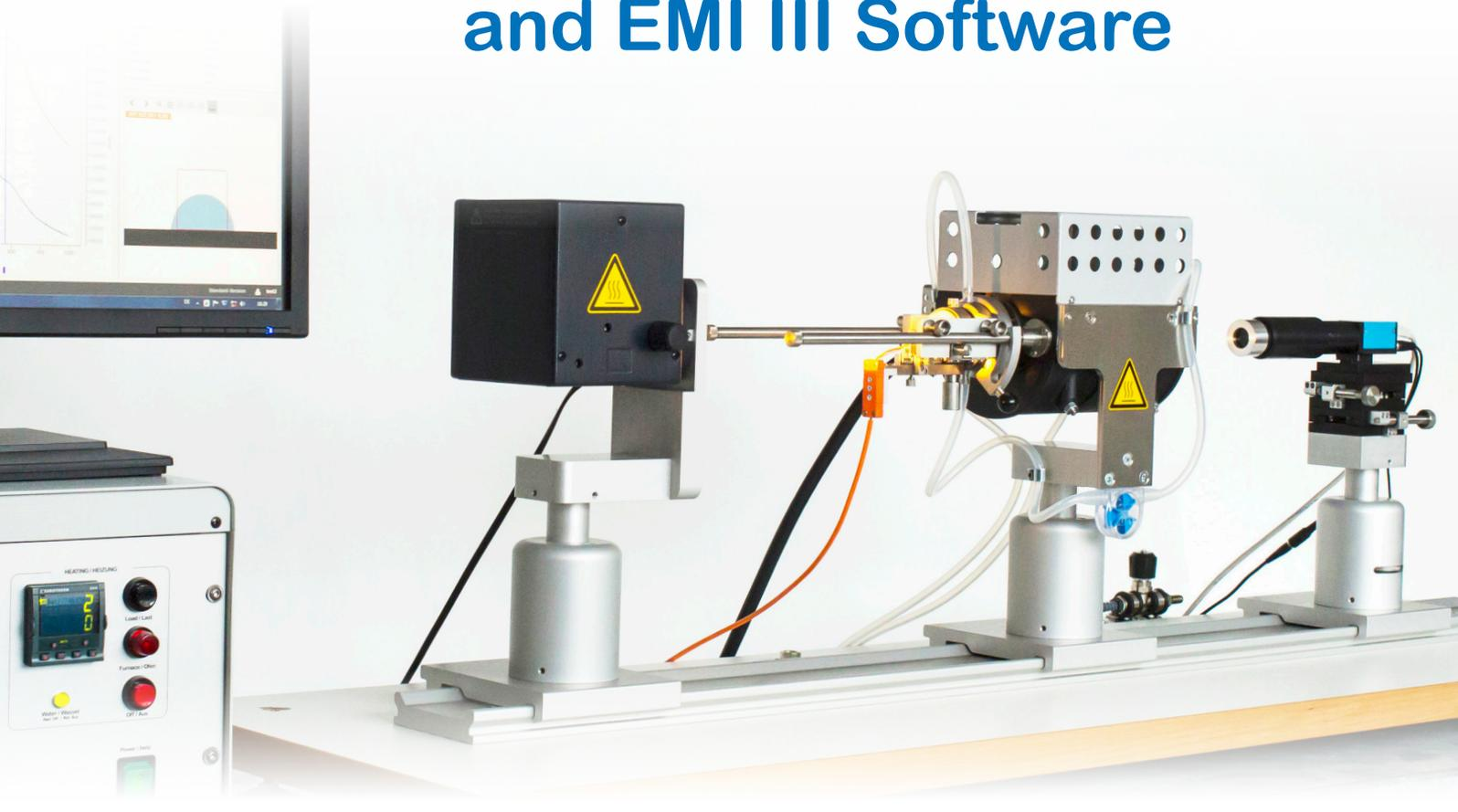
Determine the characteristic temperatures according to international standards of ash fusibility
