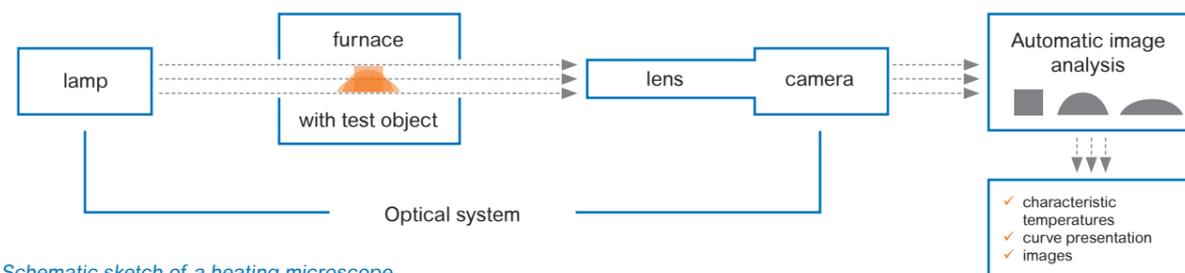
Schematic sketch of a heating microscope
